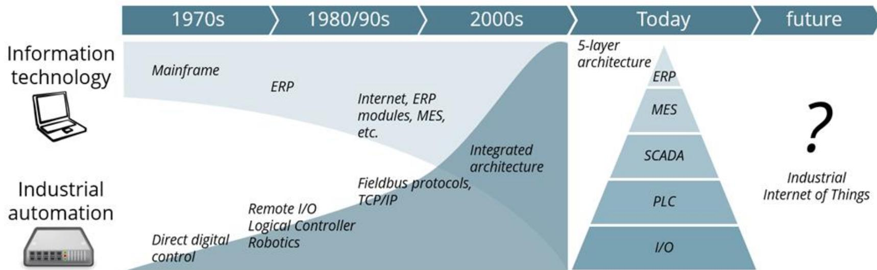
ERP = Enterprise Resource Planning MES = Manufacturing Execution System SCADA = Supervisory Control and Data Acquisition PLC = Programmable Logic Controller I/O = Input/Output signals Source: IoT Analytics
